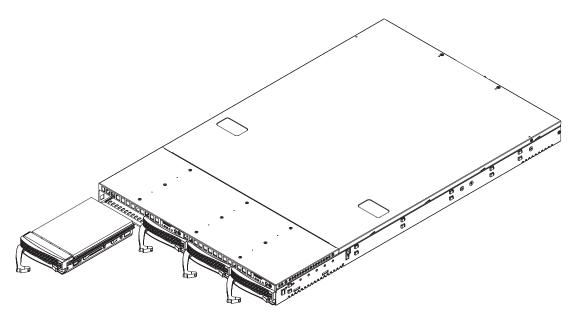
Figure 6-4. Removing a SATA Drive
